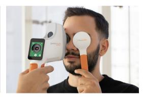
Video view for fast cameraaided alignment; continuous measurement for results in less than 10 seconds
